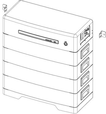
First use the fixing parts to lean against the battery where there are screw holes, and mark on the wall.
