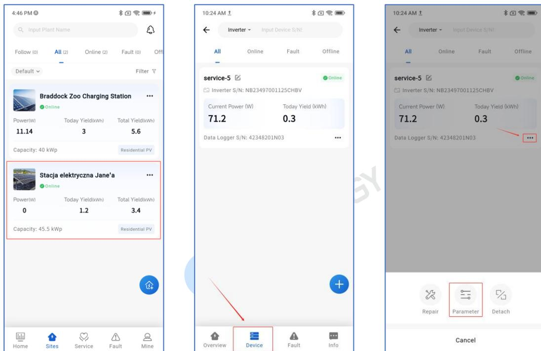
Select the parameter menu to be set in the Parameter page (such as "**Grid parameters**"), click "**Read**" to obtain the current parameters of the device, and after successful acquisition, modify the content to be set. Click "**Write**" to send the data to the device.
